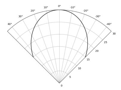
Detection distance for a 30x30cm pan of N-heptane (horizontal and vertical direction).
