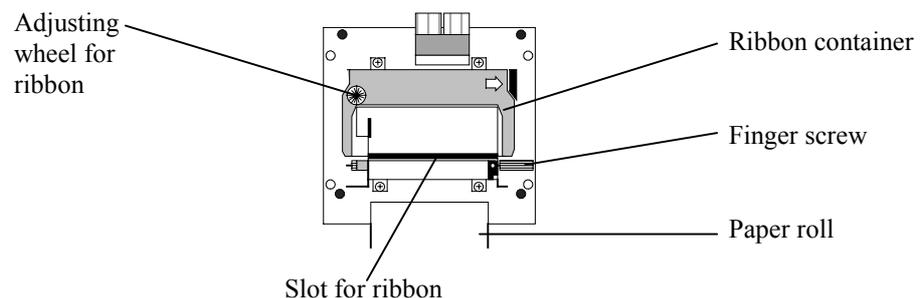
*Fig. B: Location of the finger screw on the optional printer (front view).*
