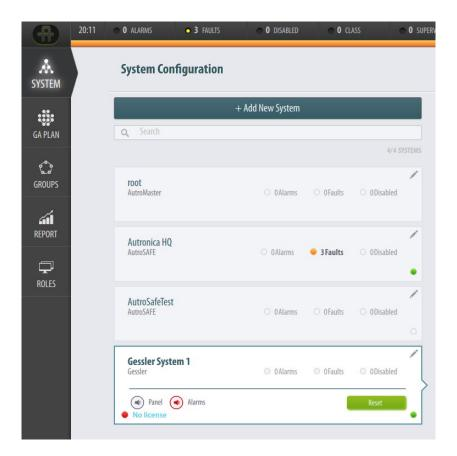
The status information for the selected Gessler system will appear in the status window in the middle of the screen. The first line shows the name of the system, the IP address and the current state (connected/disconnected).
