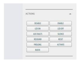
For example, the actions (DISABLE, ENABLE, LED ON, LED OFF) for a detector are shown below.
