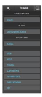
The service menu is located rightmost on the horizontal Status Bar, and includes the following submenus:
