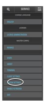
In case there is no physical keyboard connected to your AutroMaster, a virtual keyboard can be used. When the keyboard is enabled in this menu (Enable Keyboard), a virtual keyboard will appear automatically on the screen whenever a text field/dialogue box appears and the cursor iss blinking (for example, when you click the Search button). To turn off the keyboard functionality, click Disable Keyboard.
