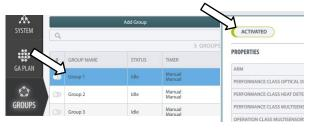
The background of the buttons will turn light grey, and the status text ACTIVATED on the rightmost button will change to DEACTIVATED when the group is activated.
