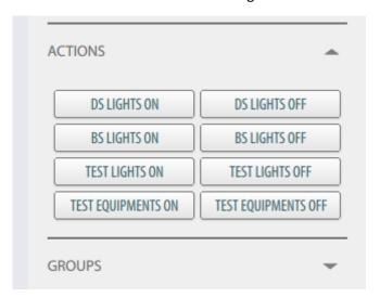
The unit status (ON/OFF) is indicated in the System tree view. For example, if Lights OC shows "false" in the status window, it will change to "true" when you select DS LIGHTS ON (as a result of the system action).
