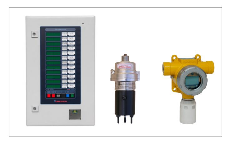
Fixed Gas Detection System OGS 2.1 is a fixed detection system for pump rooms, AC inlets (ISGOTT 5<sup>th</sup> edition) and other areas. The sensors are based on Eex D approval. Most common gas sensor types are hydrocarbon, oxygen and hydrogen-sulphide. The system can independently handle infinite number of sensors. Each alarm unit has individual display,
