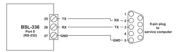
Remove the connector block from cable XJA-037. Connect the wires as described in the following table:
