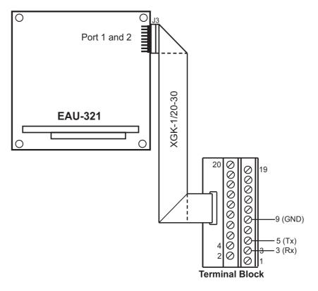
The drawing shows an EAU-321 Port 1-connection. EAU-321 Port 2 may be used with connection terminals 13, 15 and 19.
