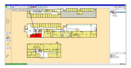
When an alarm is given, the mimic will alter to indicate the alarm location. The Detail Pane will show a flashing detector until you click the "Silence" button. The Information Pane will show the analogue value of the detector, and this information will also be marked in red in the room/area where the detector is located (providing that this is defined).
