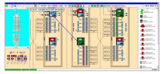
In the example below, the Secondary system is active. The symbols for the loops are coloured green and are blinking (configurable) to notify that the loops are controlled by the Secondary system.
