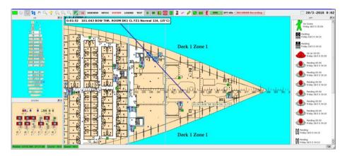
When an alarm from an fire alarm panel occurs, the screen changes so that the mimic for the detector which has given alarm is displayed. The detection zone is highlighted, and the detector which has given alarm will also be displayed, even if the detector layer is deactivated. If SMV values are configured in the mimics, AutroMaster displays colour-filled rooms/areas representing the SMV value.
