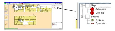
The colour of a mimic box will change to a different colour if a fault, a prewarning or an alarm situation occurs;
