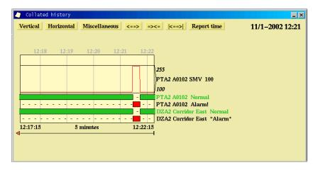
The figure shows a complete log from a point. The figure contains the detector, detection zone and the SMV value for the detector.
