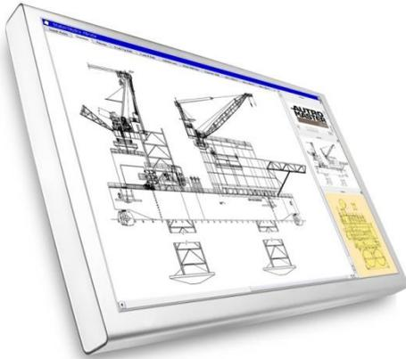
**AutoMaster** is a *remote* monitoring and control system that enables full operation of the AutoSafe Maritime Gas Detection System. All alarms, faults, inhibits, overrides and outputs can be monitored and controlled from AutoMaster.
