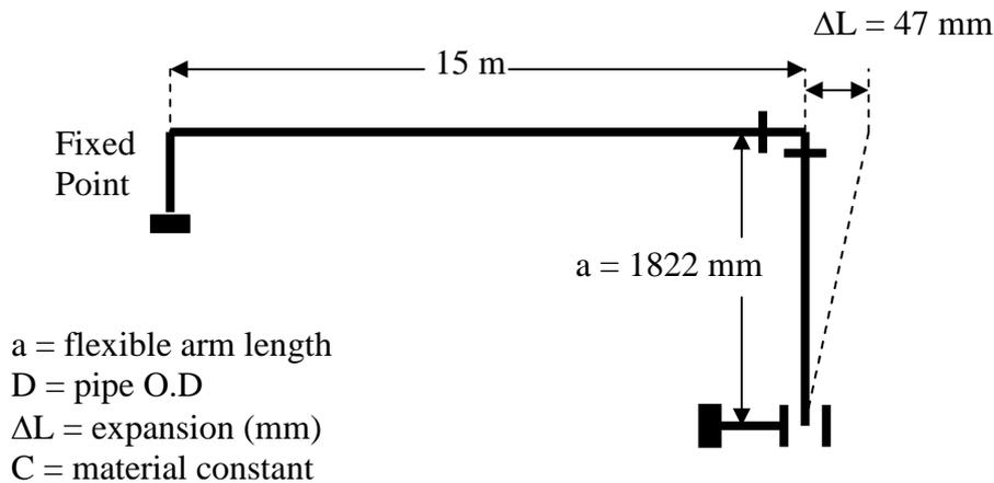
$$\therefore a = (\sqrt{D \times \Delta L}) \times C = (\sqrt{63 \times 47}) \times 33.5$$
