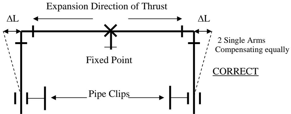
The bracket has been placed to ensure even distribution of length change, either side of the fixed point. It is not advisable to place the bracket so that the distribution is uneven.
