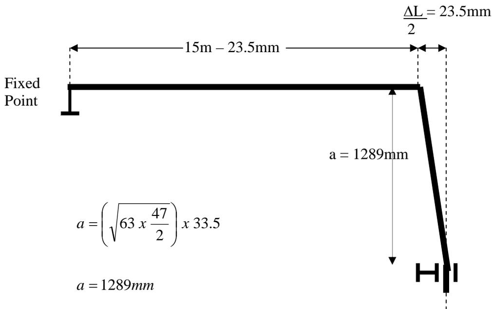
By pre-stressing the flexible arm it has been possible to reduce the arm length, and the pipe can now expand and allow (a) the flexible arm to straighten and to relieve the pre-stress.
