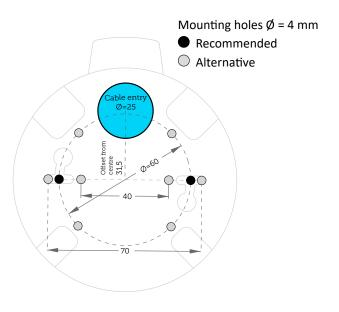
A template in scale 1:1 is found on the bottom of the protector base's packing.
