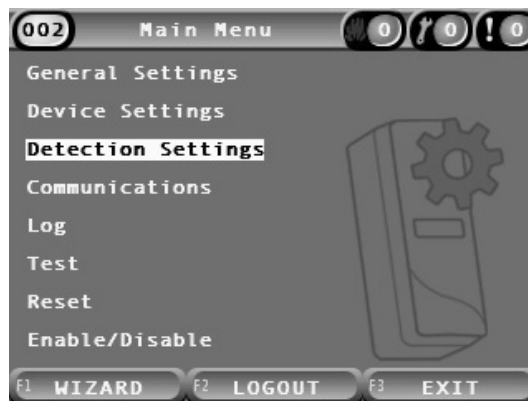
Figure 25: Access level 4 Main menu
