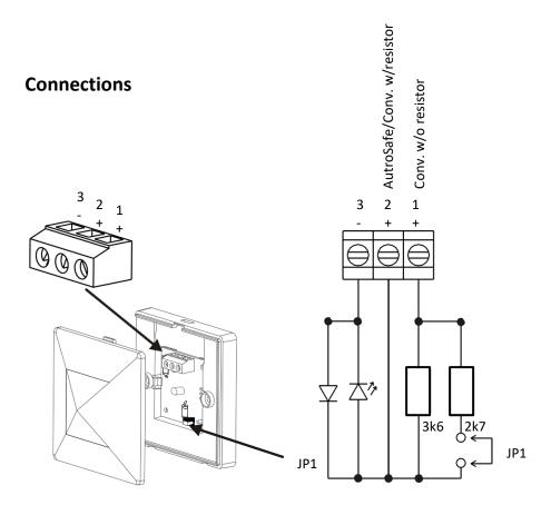
When controlled from detectors with built in current limiter (applies for BS-100 systems, AutroSafe/Autroprime and conventional heat detectors BD-2X/T):
