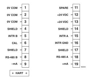
Figure 15—Wiring Terminal Identification for AutroPath HC800 Receiver without Relays
