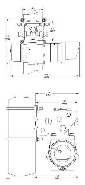
Figure 4—Mounted Dimensions of AutroPath HC800 Transmitter in Inches (cm)
