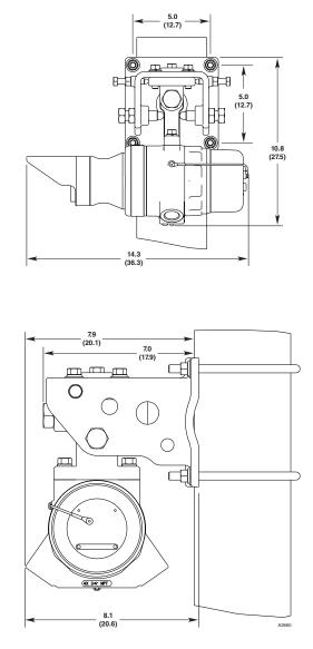
Figure 5—Mounted Dimensions of AutroPath HC800 Receiver in Inches (cm)
