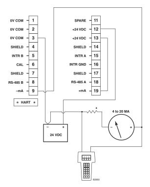
\*TOTAL LOOP RESISTANCE = 250 OHMS MINIMUM, 600 OHMS MAXIMUM. NOTE: SHIELDED CABLE RECOMMENDED (REQUIRED FOR ATEX).
