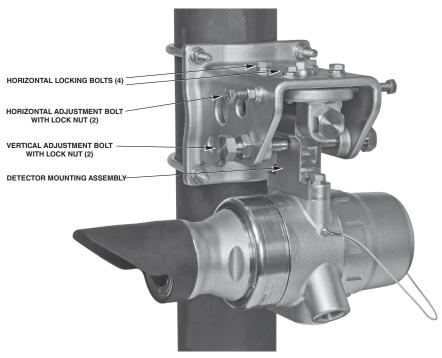
Figure 23—AutroPath HC800 Mounting and Alignment Bracket (Receiver Module Shown)
