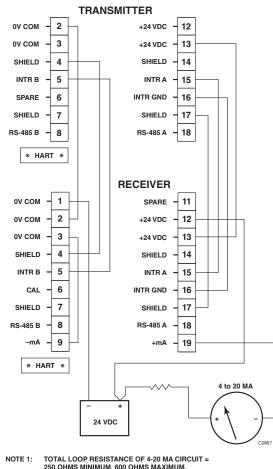
NOTE 2: NOTE: SHIELDED CABLE RECOMMENDED (REQUIRED FOR ATEX). CAUTION: DO NOT CONNECT THE COMMUNICATION LINK "INTR GND" TERMINAL TO POWER SUPPLY COMMON OR ANY OTHER GROUND CONNECTION.
