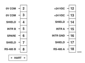
Figure 12—Transmitter Wiring Terminal Identification
