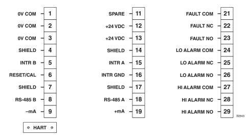
Figure 13—Wiring Terminal Identification for AutroPath HC800 Receiver with Relays
