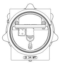
Figure 14—Terminal Strip Located Inside Wiring Compartment
