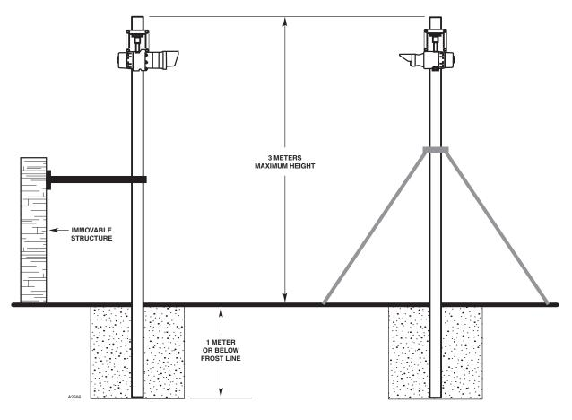
NOTE: INSTALLATIONS NEAR MAXIMUM HEIGHT TYPICALLY REQUIRE BRACING TO ENSURE NO MOVEMENT OF THE HC800 DETECTOR.
