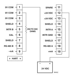
NOTE: THE HART HANDHELD DEVICE CAN BE CONNECTED EITHER TO THE HART TERMINALS OR ACROSS THE LOAD RESISTOR.
