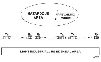
Figure 6—Proper Order of Modules for a Multiple System Installation
