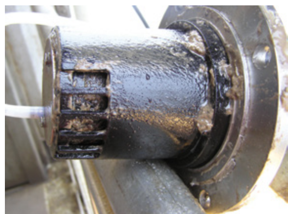
Traditional open point-IR gas detector after only a few weeks in a shale shaker environment
