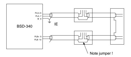
If there are break-outs from the main loop (to make local small loops that return to the same break-out box), care shall be taken to avoid local closed loops. See the figure below.
