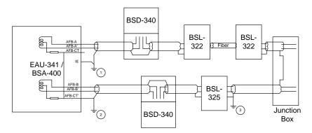
The cable shield is referenced to earth at Earthpoint 2 according to the guidelines above. Through the BSD-340 the shield is continued. There's a galvanic isolation in the Booster (BSL-325) that makes the cable (on the right side) floating. To avoid this, the Center Tap of the transformer of the AutroFieldBus (internal in the BSL-325) is terminated to the local Earth at Earthpoint 3.
