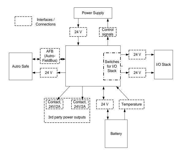
The Power Cabinet BP-405 supplies a maximum of 5A, of which 3A is available for the fire detection system. 2A is used for the charging and maintenance of the battery. Note that the maximum load for each output (A1, A2, B1, B2, C1, C2) is 2A.
