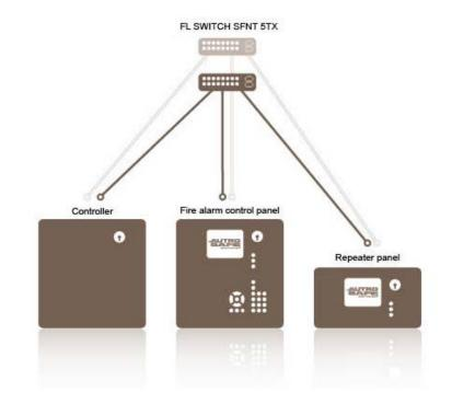
A simple network system. The transmission length between the panels and an Ethernet switch does not exceed 100 meters.
