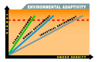
By choosing a sensitivity setting that suits the environment, it is possible to achieve an accurate and reliable system, providing the optimal detection, whilst virtually eliminating false alarms.
