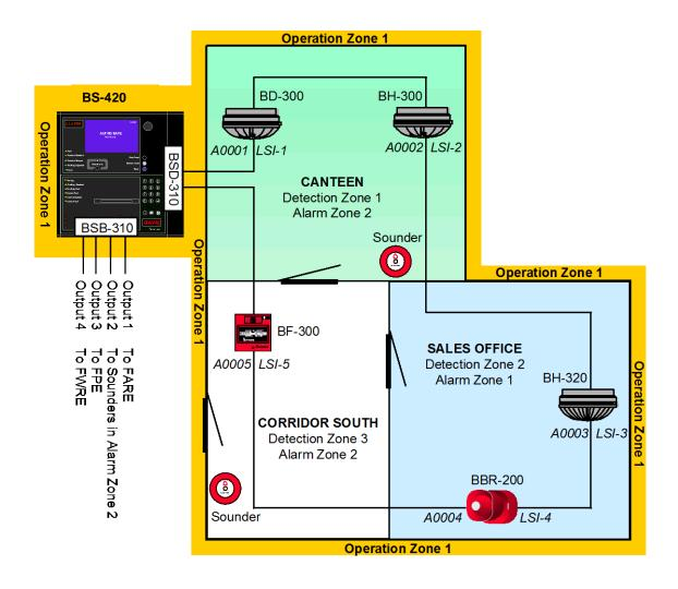
The building is divided into three sections, the CANTEEN, the SALES OFFICE and the CORRIDOR SOUTH, each section defined as a *Detection Zone* (1, 2 and 3).
