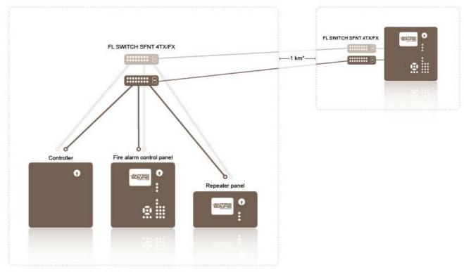
The transmission length depends on the fibre optics cable specifications.
