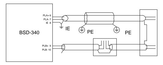
PE will make earth loops as they are terminated at multiple points, however the loop area will be narrow or closed as the armour will be close to the frame or earth. It is essential that the armour is kept on the same equipotential around to avoid EMC problems or large current flow in the PE. PE may be connected through glands to the junction boxes to form a continued protective armour or shield. Still the internal shield and IE shall be kept isolated from the PE.
