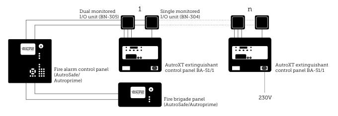
The AutroXT extinguishant control panel BA-51/1 is connected to the AutroSafe 4 / Autroprime fire alarm control panel via two I/O units, each panel covering one zone.
