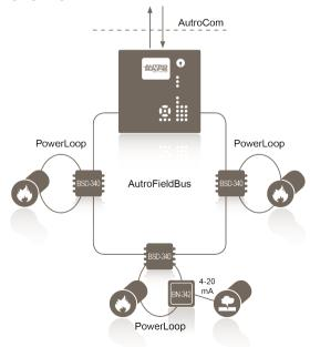
Note: All PowerLoop cables must be shielded.
