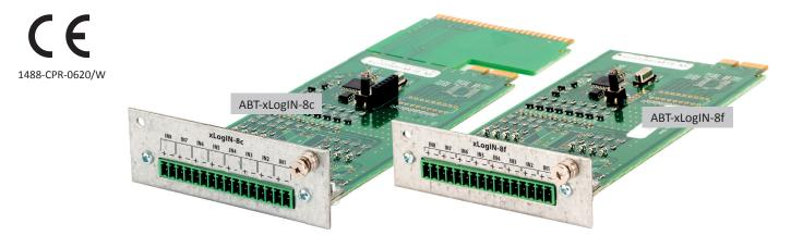
The logical input card for a function or control slot has 8 control inputs which may receive signals from other systems in order to trigger a desired reaction of MULTIVES system. Inputs of an ABT-xLogIN-8c/f card offer two modes of operation: contact mode (short / open contact) and monitor mode in which in addition to contact mode function, short circuit and opening of the cables connected to the card are detected.
