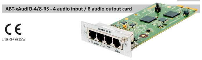
This audio intput/output card is destined for a function slot of ABT-CU-11LCD. It offers 4 line audio inputs via an RJ45 conector as well as 8 symmetrical outputs via an RJ45 connector for leading out audio signals to the external devices or amplifiers of the MULTIVES system. The card is also equipped with an RS485 interface with the help of which the MULTIVES system can be controlled or integrated with devices offered by other producers.
