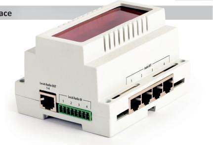
The ABT-ISLE allows integration with other interfaces and different devices using RS485 protocol. It's also audio cable splitter from 1 x RJ45 consisting 4 analog audio channels coming out from Audio Out on CU to 4 x RJ45 where each of RJ45 includes 1 audio channel for amplifier input. Unit housing is designed for rack rails TH 35. Address of the ABT-ISLE must be unique and can be set by dedicated Addressing POT (16 addresses 0-F). First module in chain has to have address 0.
