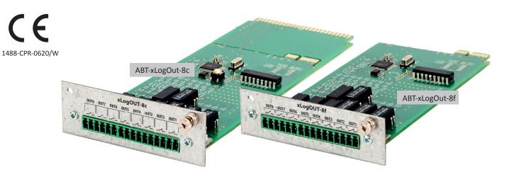
The logical output card has eight fully programmable relays which can be used for acknowledge the various states of the Multives outside to other systems. The channels from 1 to 4 are equipped with NC and channels from 5 to 8 with NO type of relays.
