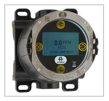
All electronics are enclosed in an explosion-proof aluminum or stainless steel housing. The display unit is used with a single detector that may be either coupled directly to the AV10, or remotely located using a sensor termination box. The AV10 features non-intrusive calibration. A magnet is used to perform calibration as well as to navigate the AV10's internal menu.
