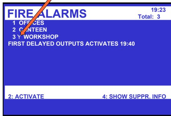
After pressing the ENTER button and selecting the delayed action zone, you can;
