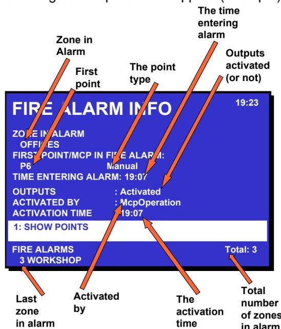
Detailed zonal information will be available. In the *example* above you can view the zone in alarm, the first point in fire alarm, the time entering alarm, the activation state of outputs, what triggered the alarm (for example, Manual Call-point operation) and the activation time. You can also move directly to SHOW POINTS (press digit 1).
