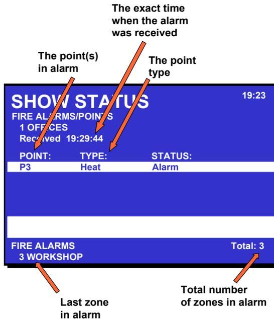
Here (*in this example*) you can view the points in alarm and the type of point (detector type, manual call point). The arrow buttons are used to move up and down in the list of points.
