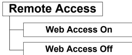
This command allows you to access a web site where you can perform system service functions from a computer via the Ethernet connections.
