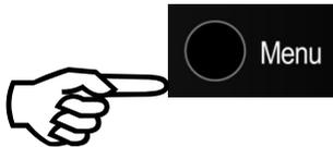
To enter the *Menu Mode* from operation mode or the panel's idle state, the Menu button must be pressed. The menu has 5 different menu selections, including SHOW STATUS, DISABLE, ENABLE, SYSTEM and SERVICE.
