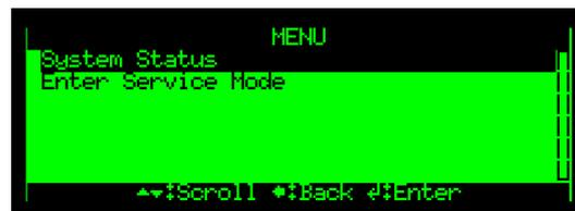
If the panel is set to access level 2 (the key is turned clock-wise), six different menu selections are shown in the display, including *System Status*, *Disable*, *Enable*, *Show Unit Properties*, *Report* and *Enter Service Mode*. If the panel is set to access level 3 (Service Mode is entered using a password), the seventh menu selection *Exit Service Mode* is shown in the display.
