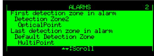
The total number of detection zones (in this example, 2) in alarm state is shown in the upper right corner of the display.
