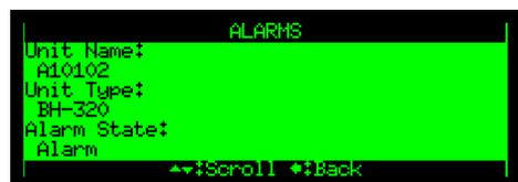
A black mark on the vertical scrollbar on the right side of the display indicates that you can scroll downwards (or upwards) to reveal more information. Note that this is not indicated on the illustration.
