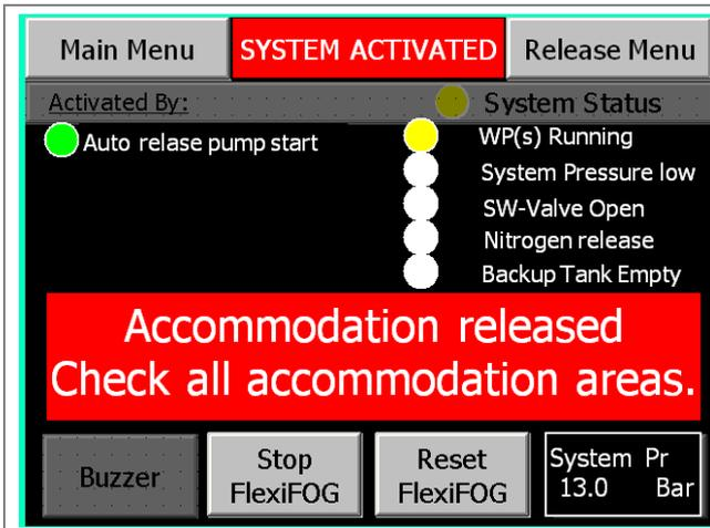
When activated, the screen will display which fire zone is released.
