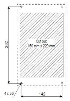
Cut out for flush mounting Dotted line - Outer dimension panel
