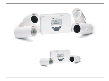
Both the detector heads, Transmitter and Receiver, have integrated alignment thumbwheels for ease of alignment. Using these thumbwheels provides a smooth and repeatable alignment process. The detector heads have up to 10 degrees of adjustment in both planes. For further adjustment, a bespoke Adjustment Bracket is available, which offers up to 180 degrees movement in both planes, as well as a full 360-degree rotation.
