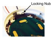
mounting (with a pair of cutting nippers or similar), the detector head will be locked.
