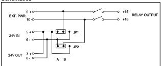
Note that the 7A output load is only permitted if external power is fed to terminals 9 and 10. The jumpers JP1 and JP2 should then be removed. If fed from external 24V, through jumpers JP1 and JP2, the maximum current output is derated to 1A.
